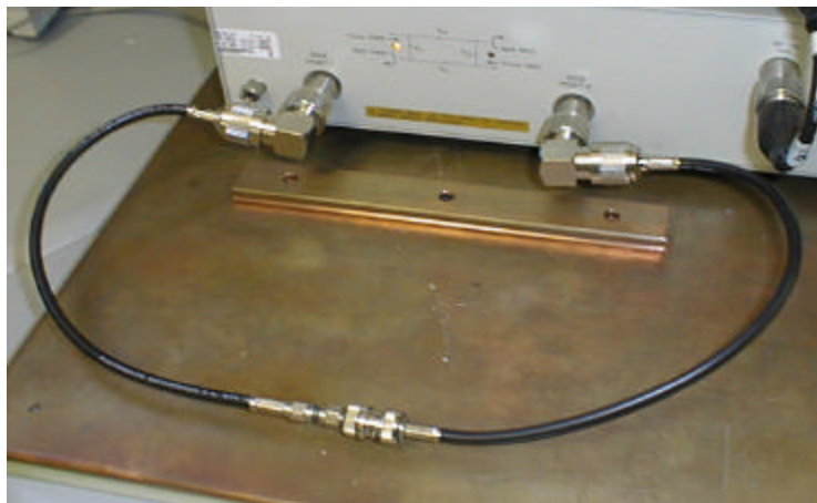
24 Figure D.1 – Coaxial lead attenuation calibration
